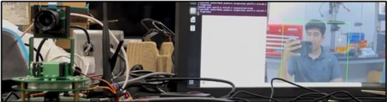
Fig. 6. Representative live tracking frame showing person detection and active target selection.
