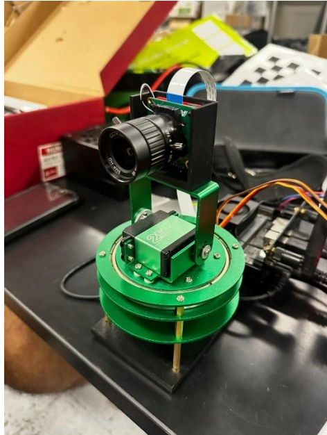
Figure 2. Final AI camera tracking prototype prepared for BillyBOT integration.
